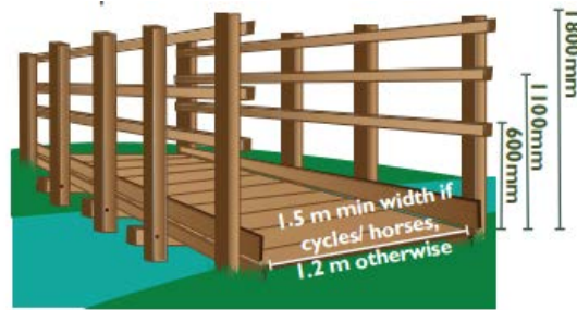
Fig. 3b – Typical bridleway bridge design
